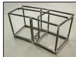
Welded and ground Frame ready for powder coat
