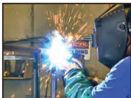
Frames are welded together
