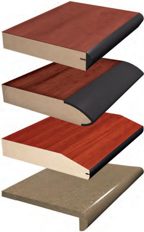
**LAMINATE WITH SAFEGUARD™** Choose from a broad range of colors, textures and patterns. We supply laminates from all the major manufacturers. The high pressure laminate is permanently bonded to an industrial grade 45 lb. density particle board core for strength. The work surface is finished with our durable Safeguard Edge.
